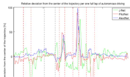
Figure 11: Relative deviation from the center of the trajectory per one full lap.
