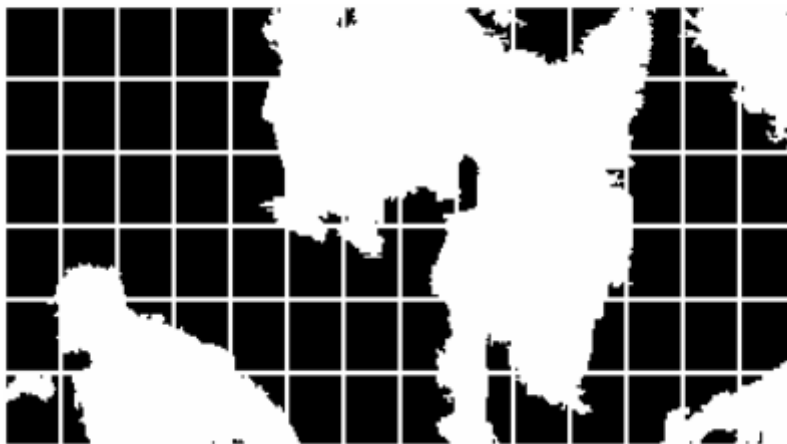
b) camTS binary image with foreground pixels; original grid of 83 cells; size of each cell is 25 \times 30 pixels
