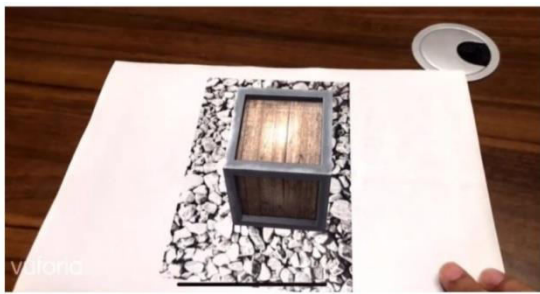
Fig.1. Vuforia image tracking
