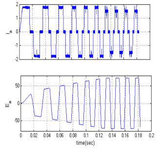
Fig.11 Stator current and emf.
