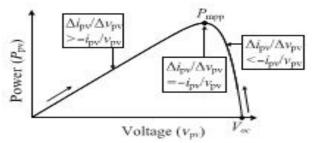
. Fig.3. Illustration of INC-MPPT with SPV array  $P_{p\nu} \!\!-\!\! V_{p\nu} characteristics$
