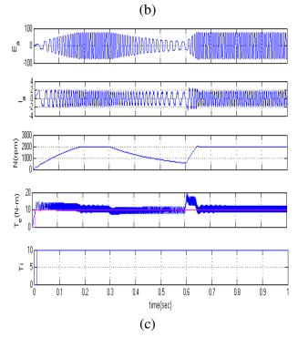
Fig.7 Dynamic performances of the proposed SPV array-based zeta converter-fed BLDC motor drive for water pump. (a) SPV array variables. (b) Zeta converter variables. (c) BLDC motor-pump variables.
