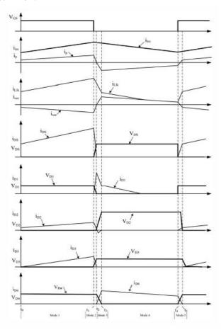
Fig.4. Key theoretical waveforms of the proposed converter.
