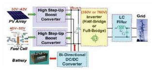
Fig.1. Diagram of a single-phase renewable energy grid-connected system
