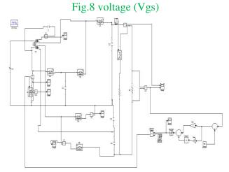
Fig.9 simulink model of step-up dc-dc converter with closed loop control
