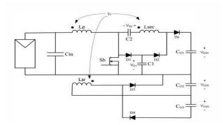
Fig.2. Proposed High Step-Up Converter.
