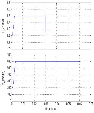
Fig.11 Voltage and Current wave forms with sudden decreasing load
