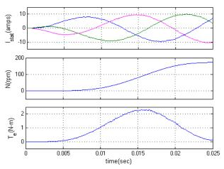
Fig.14 Stator current, Speed, Torque characteristics of the induction motor
