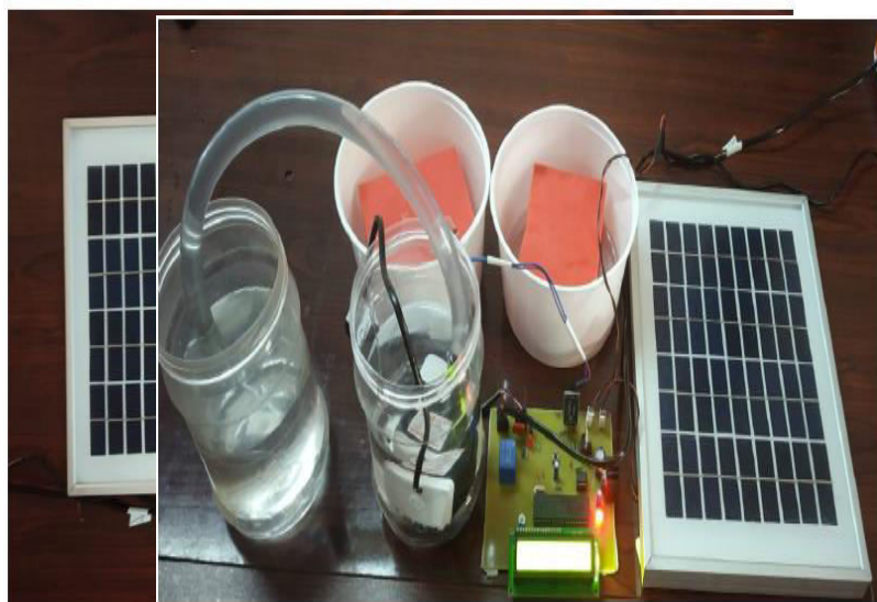
Figure.5. Hardware setup of the proposed irrigation system using solar power
