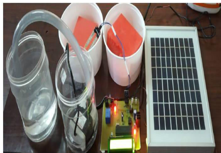
Figure.6. Operation of the Hardware setup of the proposed irrigation system using solar power under soil dry condition
