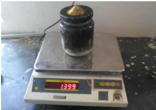
Fig. 4.2: Testing on le-Chatelier flask
