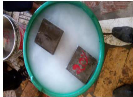
AID CURING OF CONCRETE CUBES
