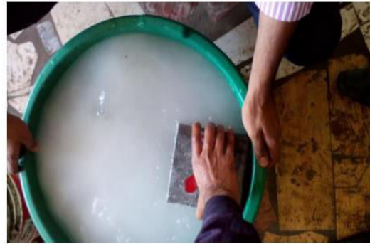
ALKALINE ATTACK TEST OF CONCRETE CUBES
