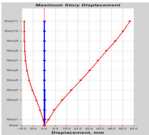
Maximum storey displacement for structure-3
