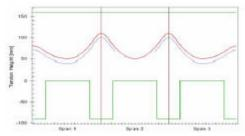
Fig. 4. Tendon profile for the slab with drop
