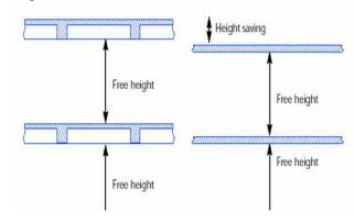
Traditional R.C.C. design PT slab design Fig. 1. Height comparison of R.C.C. & PT slab design
