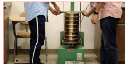
Figure-5: Pouring the soil sample on sieves and vibrating on sieve shaker
