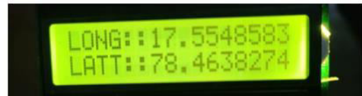
Fig 14 : The display of the GPS Values sent to the registered numbers
