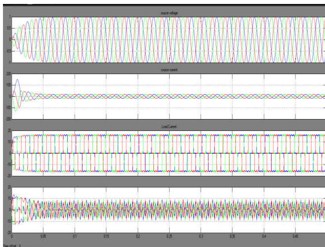
Fig.16 shows the simulated waveforms of proposed system like Source voltage, source current, load current and compensation currents with fuzzy logic controller
