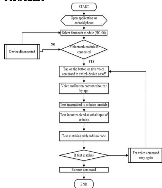
Figure8. Flow chart of the system operation
