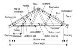
Slope is the measure of how "steep" a roof is. For example, if a roof is "4 in 12", the roof rises 4 inches for every horizontal run of 12 inches. The pitch of the roof is a big factor in determining the kinds of materials that can be used and the longevity of the roof. Usually, a steeper roof (higher pitch) will last longer due to its better drainage capabilities. Top Chord - Main member of a truss running along the underside supporting the decking.
