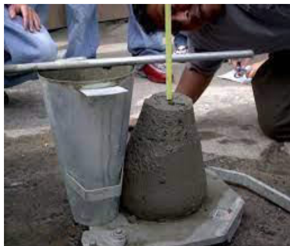
Fig. 2: Slump cone test subsidence.
