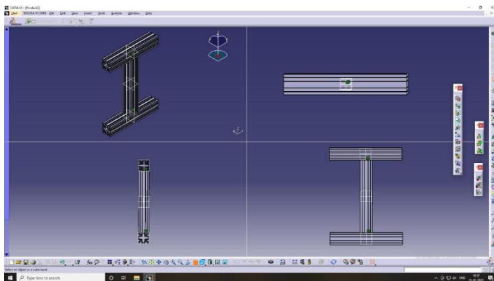
Fig.5. Assembly model of I - section portable 3d printer
