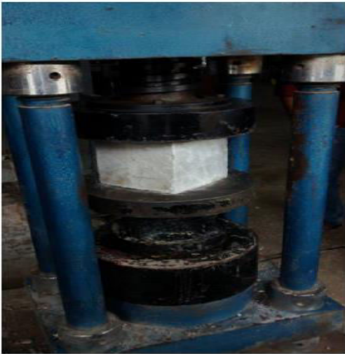
Figure shows Testing of cubes for compressive strength
