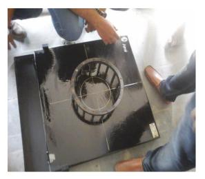
Fig: 4.2 J - ring test Apparatus
