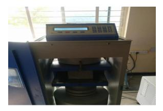
Fig: 7.2 Compressive Testing of SCC Cube Using Digital Compression Testing Machine
