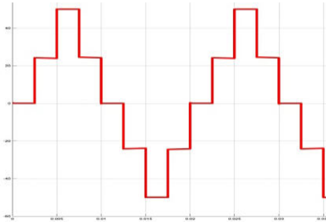
Fig.1 (c) output voltage of five level inverter.
