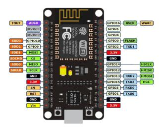
While writing GPIO code on NodeMCU, you can't address them with actual GPIO Pin Numbers as shown in Fig.4. There are different I/O Index numbers assigned to each GPIO Pin which is used for GPIO Pin addressing. Refer following table to check I/O Index of NodeMCU GPIO Pins – GPIO Pin I/O Index Number
