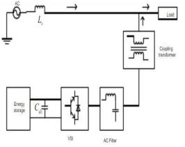
Fig.2. Single line diagram of DSTATCOM
