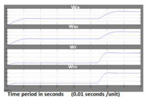
Fig.14.Matlab/Simulation of fuzzy Average value of the active weight components in-phase to the PCC voltages (wa), total active weight component (was), average value of the reactive weight components in-phase to the PCC voltages (wr), and total reactive weight component (wrs)
