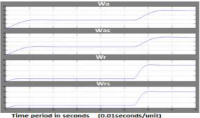
Fig.10.Matlab/Simulation of Average value of the active weight components in-phase to the PCC voltages (wa), total active weight component (was), average value of the reactive weight components in-phase to the PCC voltages (wr), and total reactive weight component (wrs)
