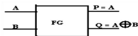
Fig 1.1 Block Diagram of Feynman Gate
