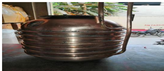
Figure: Heat Exchanger tank with copper pipe soldering.
