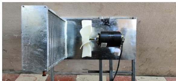
Figure: Condenser and fan fitting.
