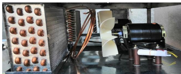
Figure: Evaporator and fan fitting.
