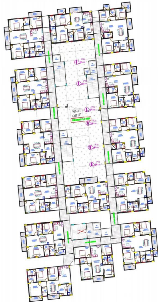
Figure 1: Plan of (G+12) Multi-Storeyed Building Loading Consideration
