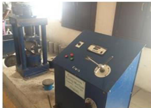
Fig 3.1.3 Split tensile set up in CTM
