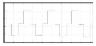
Fig.10 shows the simulated output waveform voltage across switched capacitor
