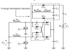
Fig. 2 Proposed high step-up converter
