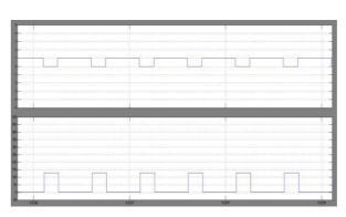
Fig.9 power switch S2 gating pulse and output voltage
