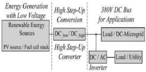
Fig .1: Block diagram of the whole system
