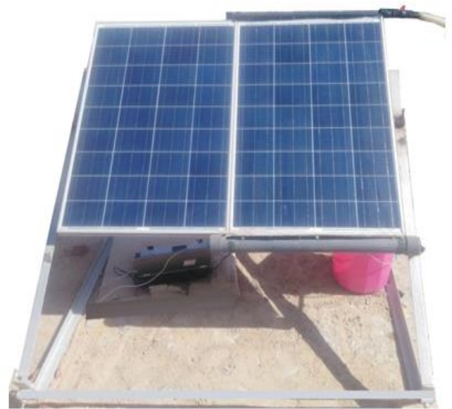
Fig.3 PV system experimental (one PV module With free front flow cooling and the other without cooling)
