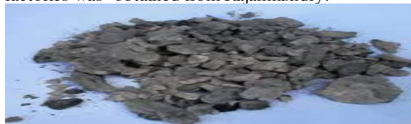
Fig :1Waste paper sludge ash
