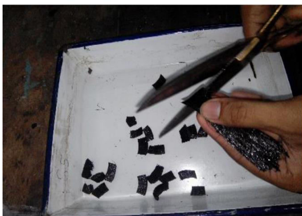
Figure 3.7 Cutting of coated fiber.
