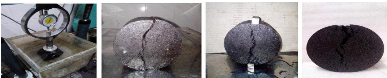
Figure 3.10 Loading and failure pattern of indirect tensile strength test.
