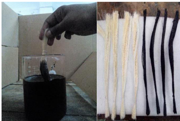
Figure 3.5 Coating of emulsion on fiber.
