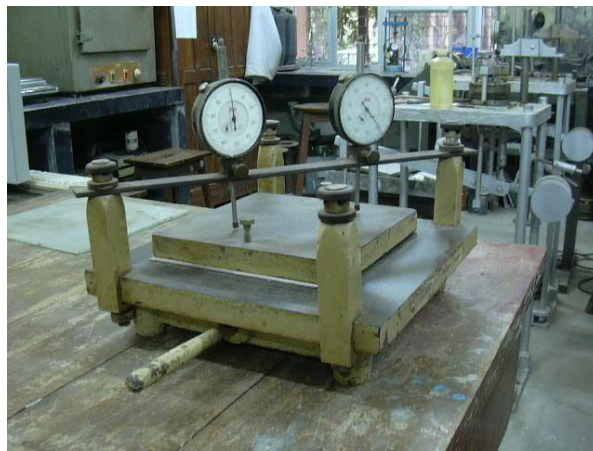
Fig 2.12 Thickness measurement apparatus
