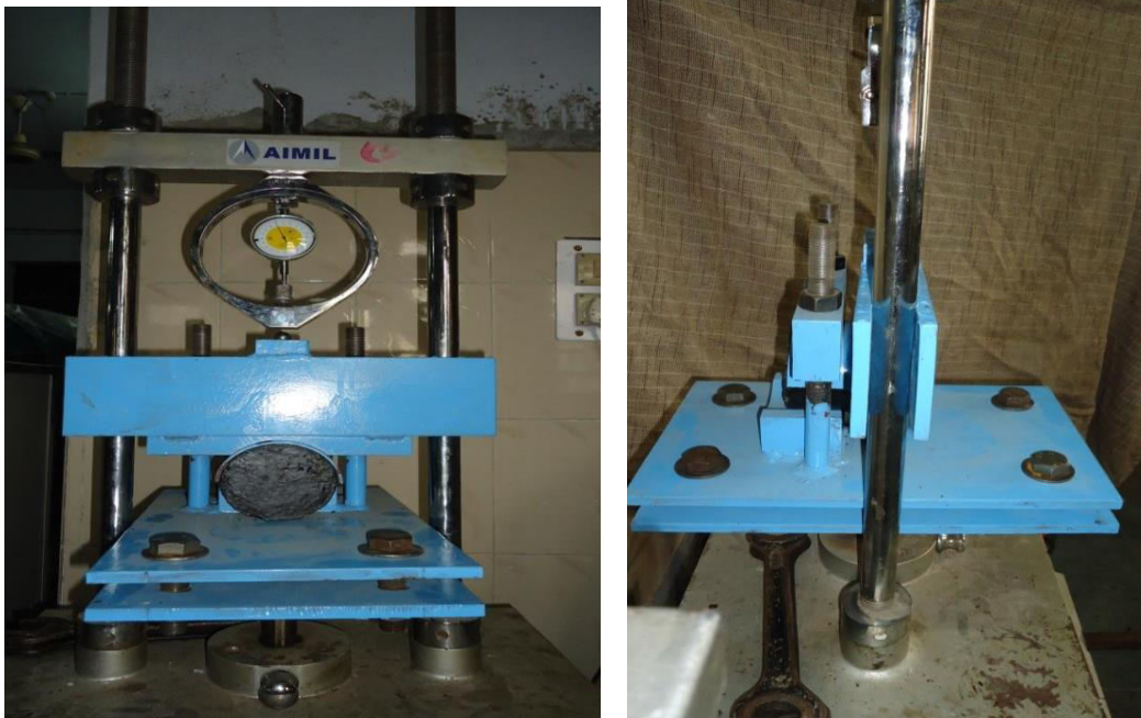
Figure 3.7. Photographs of the Shear-Testing model no. 1
