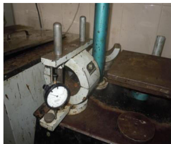
Figure 3.7 Breaking Head of Marshall Apparatus
