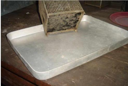
**Fig. 3.8 Drainage of CRMB 60 binder sample**
