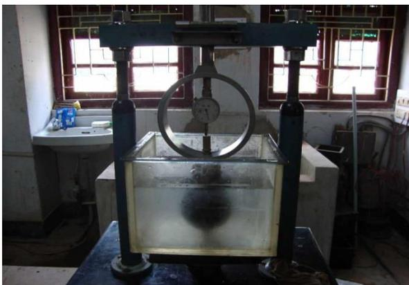
**Fig. 3.9 Static indirect tensile test in progress**
