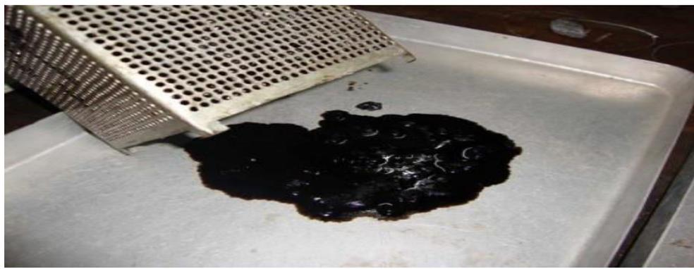
**Fig. 3.5 Drainage of 80/100 bitumen sample**
