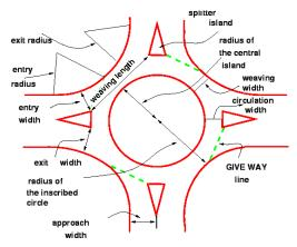
Fig 1: Design elements of a rotary
