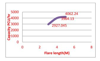
Based on the results, from the following graph 1 we can observed that the capacity of roundabout is increased with increase in entry width
