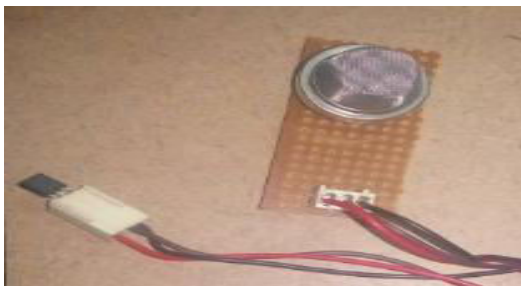
Fig 6.5 Temperature and Smoke sensor
