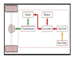
FCEVs also called as the fuel cell electric vehicles. FCEVs driving component is electric
