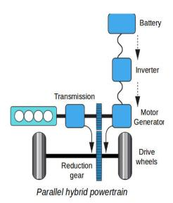
Both the internal-combustion engine and the electrical generator can send torque to the driving wheel simultaneously or sequentially in a parallel hybrid power train. A typical hybrid power train architecture for a rear-wheel drive (RWD) vehicle places an electric motor between two clutches
