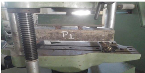
Fig 3 testing of specimens for flexural tensile strength
