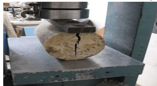
Fig 2 testing of specimens for split tensile strength
