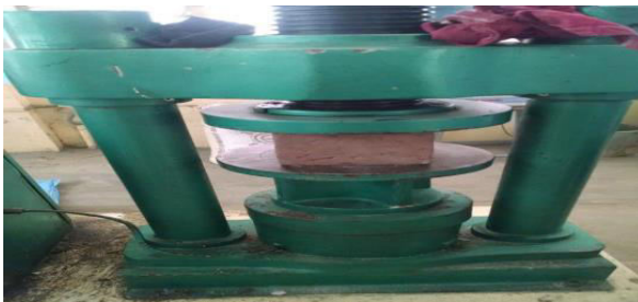
Fig 1 – testing of cubes for compressive strength
