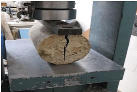
Fig 2 testing of specimens for split tensile strength
