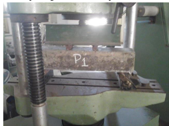
Fig 3 testing of specimens for flexural tensile strength
