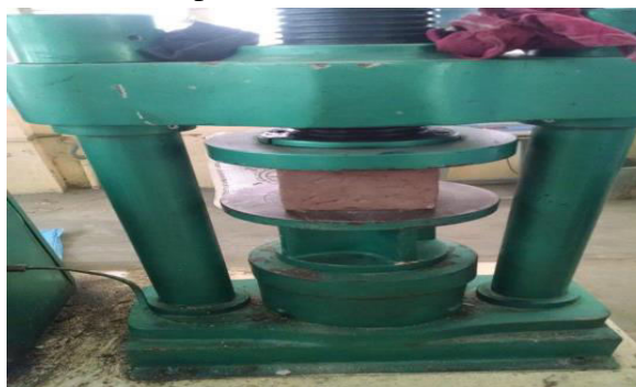
Fig 1 – testing of cubes for compressive strength
