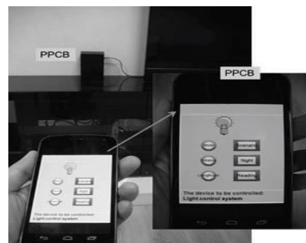
Fig.3.6 Pointing to the PPCB of the lighting control system (at this point, the states of all lights are powered off).
