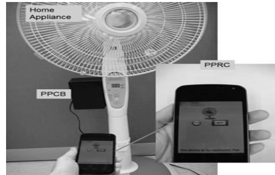
Fig.3.5 Pointing to the PPCB of the fan and pressing the “Power” button (the state of the fan is powered on in normal mode and a moderate wind speed).
