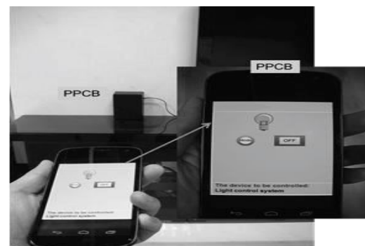
Fig.3.6 Pointing to the PPCB of the lighting control system (at this point, the states of all lights are powered off).
