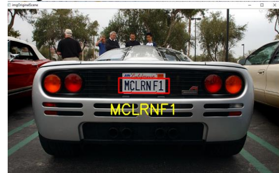
Fig (3) detecting and extracting number plate and showing output
