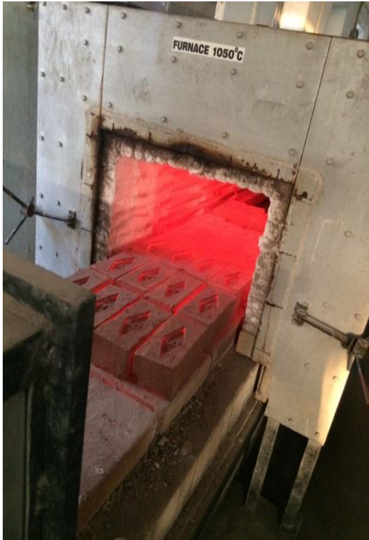
Figure5. Bricks in the furnace after heating
