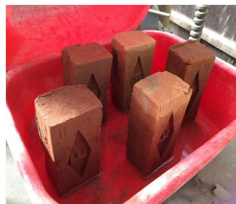
Figure7. Bricks in efflorescence test
