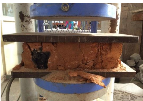
Figure 6. Compression test on burnt brick
