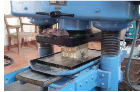
Fig. 6.1 Compressive Strength Test
