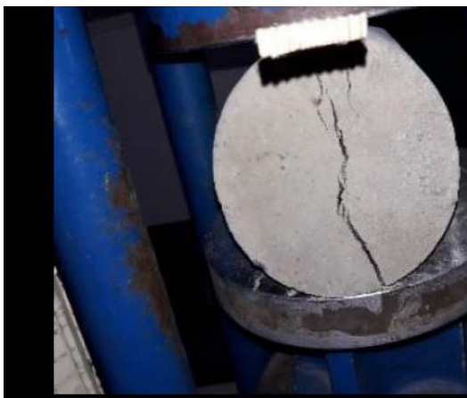
Fig.6.4 Split tensile strength test
