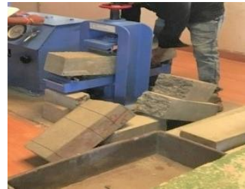
Fig 3.3 Flexural strength test setup
