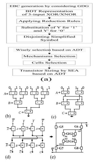
Fig. 6: (a) SCDM process for designing efficient three-input XOR/XNORs. (b)
