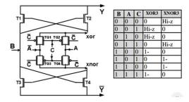
Fig 2: BC2 circuit and input and output values.
