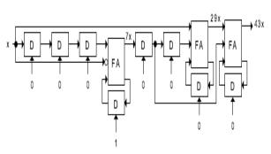
Figure 4: Bit-serial realization of shift-adds implementation of 29x and 43x given in Figure 2(c).
