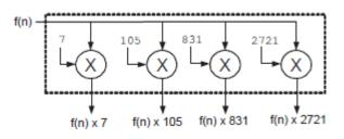
Figure 1(a): A multiplier-based MCM example
