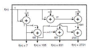
Figure 1(b): A multiplierless-based MCM example
