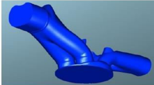
Fig.2. Perspective view of the combustion chamber geometry layout with 4-valves (bottom view)
