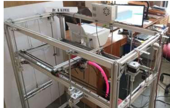
(a) View of the outer frame architecture in a 3D Printer
