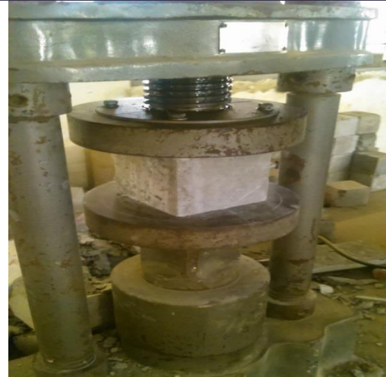
Figure: Testing of Cube Specimen in CTM Table Compressive Strength of Various Concrete Mixes with Replacement of Fine Aggregate over Waste Foundry Sand at Different Ages
