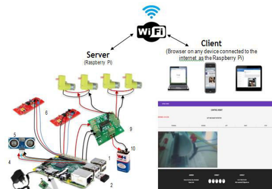
Figure 2 The initial block diagram for IOT Robot
